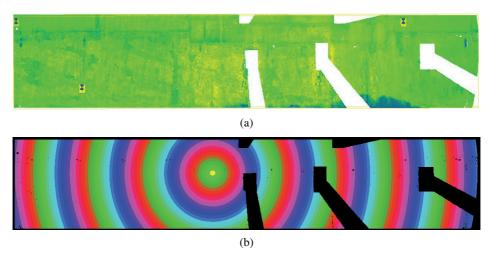
Fig. 4. Concentric nature of the distribution of the influences of the beam incidence angle and scanning distance on the recorded beam reflection intensity values: a) scan of the slurry wall in intensity colors, b) distribution of influences of geometrical factors (incidence angle, distance), a 10 cm step along the measured wall, centre: projection of the center point of the scan
