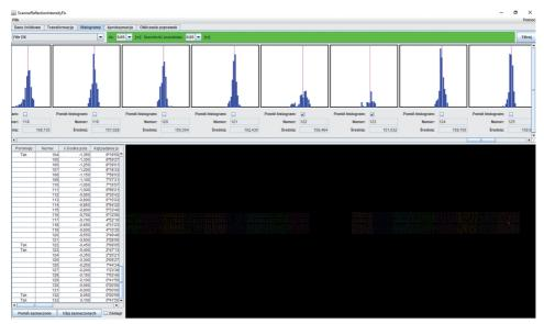
Fig. 10. Example of histogram distribution analysis of intensity values for 10 by 10 cm fields developed in proprietary Scanner\_Reflection\_Intencity\_Fix (SRIF) software
