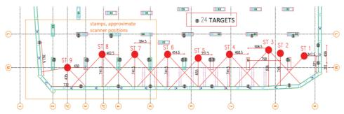
Fig. 2. Layout design of the scanner stations (ST1-ST9) and measurement targets for the selected slurry wall of the test facility
