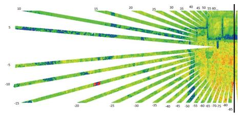
Fig. 8. Division of the point cloud into 10 cm wide stripes and distribution according to the direction of rays propagating from the center point, which is the projection of the scanner on the examined surface
