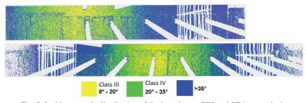
Fig. 5. Incidence angle distribution of the laser beam, ST3 and ST4 respectively
